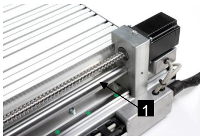
Figure 26: linear guides of the X-and Z-axis
