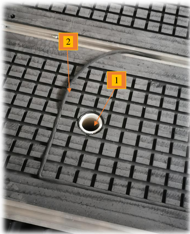
Fig. 12.4: Vacuum opening / vacuum sealing cord
