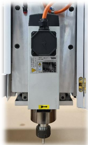
Fig. 11: HF spindle 3.5 kW
