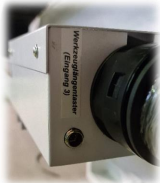
Fig. 10.4: Connection of tool length probes
