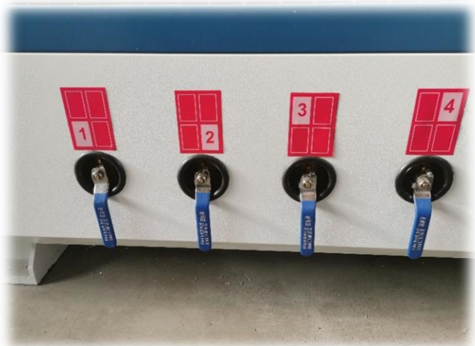
Fig.12.1: Vacuum zones and shut-off valves
