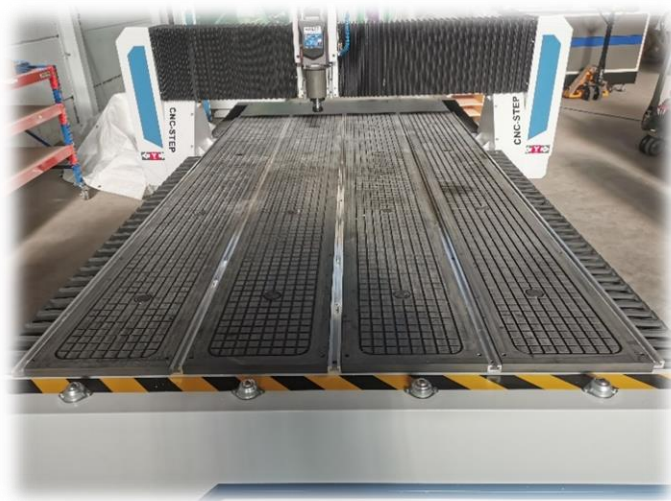
Fig.12: Machine with vacuum table and T-rails
