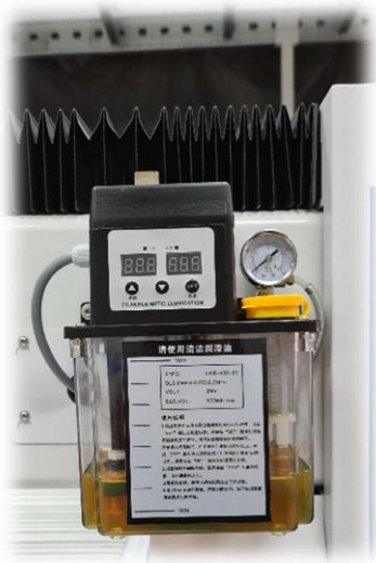
Fig. 9.1: Oil tank for central lubrication
