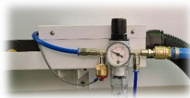
Fig. 8.4: Pressure control valve for cylinders
