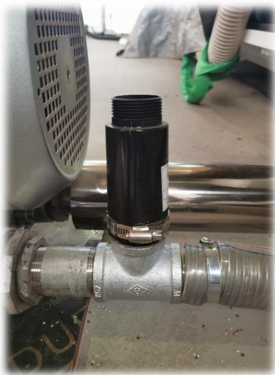
Fig. 13.2: Vacuum limiting valve
